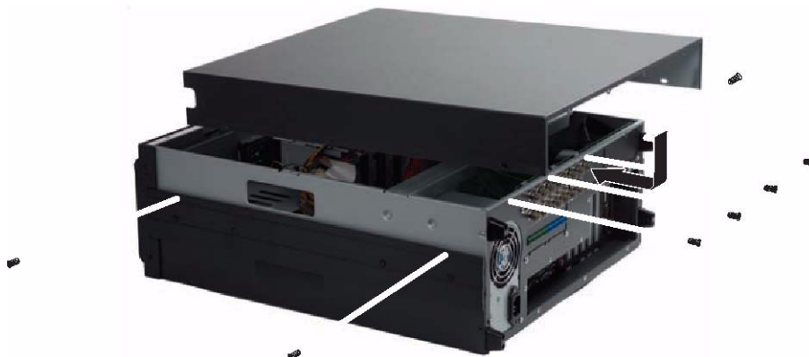
Figure 10. Replacing Chassis Cover
