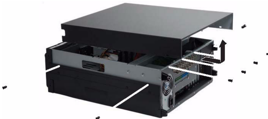
Figure 5. Removing Chassis Cover
