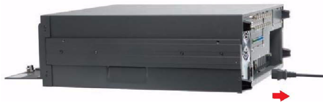
Figure 3. Removing Power Cord from DX8100
