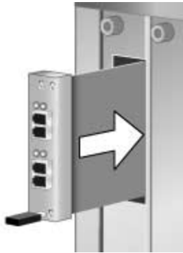
FIGURE 2-2 Inserting the HBA Into the AMC Connector
