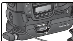
6 Open the camera USB connector cover and connect the USB cable to the USB connector.
