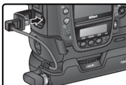
7 Pass the cable over the guide on the BL-2 battery-chamber cover.
