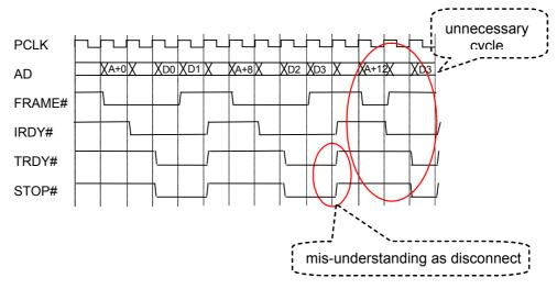
D0 ,D1,D2 are burst data; D3 is last burst data and D2 is last-but-one burst data. TRDY# and IRDY# are both asserted during D2 and D3. So data transfer of D2 and D3 is finished. But because of this restriction, VR4133 mis-interpreting data phase as if it is disconnected at D2. Therefore D3 cycle is performed again.
