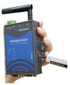
Step 2: After removing the cover, insert the SD memory card as shown.
