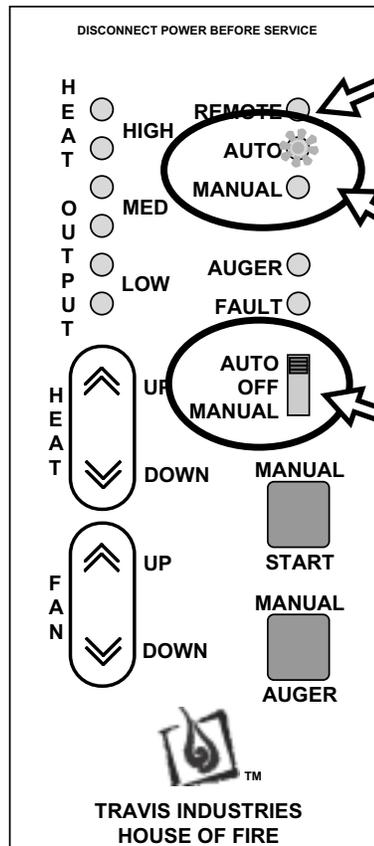
**NOTE:** if using a modulating remote, this light will come on to indicate the remote is controlling the heater.
