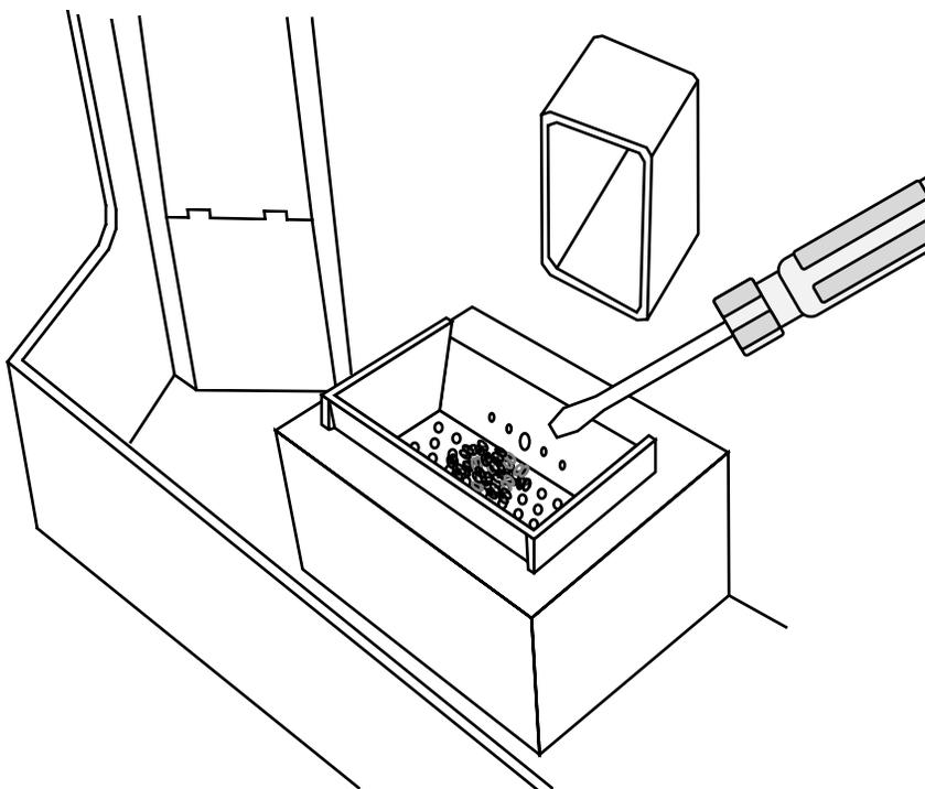
***Bi-Weekly Maintenance (or every 10 bags of pellets)*****Clean the Heat Exchange Tubes**
