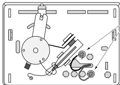
Expose 1/2" of wire and attach to these two posts.
