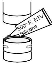
Seal each vent section by injecting a liberal amount of 500° F. RTV silicone into the gap between sections.
