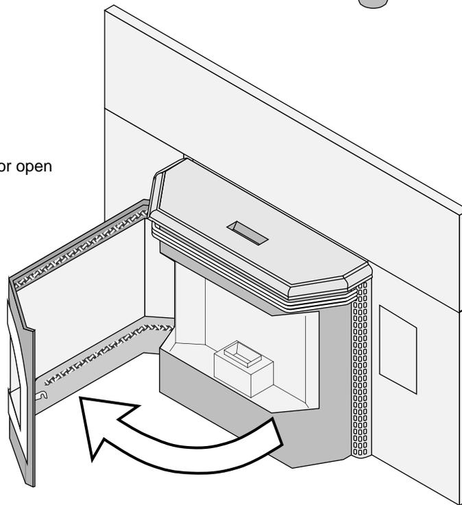
**Bi-Weekly Maintenance (or every 10 bags of pellets) - Continued****Check Ashbox, Ashpan, Dispose Ash If Necessary****Removing the Ashbox**
