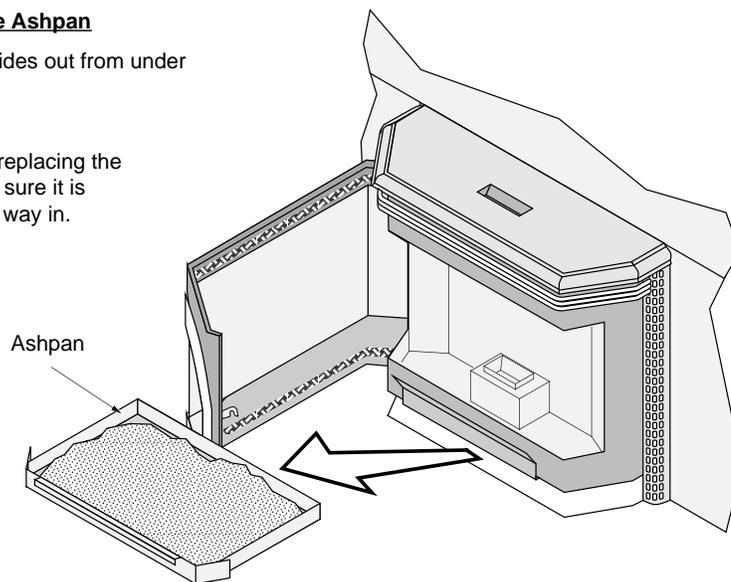
**Disposal of Ashes** – Ashes should be placed in a metal container with a tight fitting lid. The closed container of ashes should be placed on a non-combustible floor or on the ground, well away from all combustible materials, pending final disposal. If the ashes are disposed of by burial in soil or otherwise locally dispersed, they should be retained in the closed container until all cinders have been thoroughly cooled.
