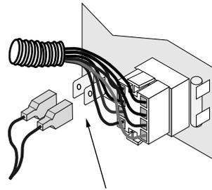
Attach the quick-connects to the two posts near the molex connector on the circuit board (orientation does not matter).
