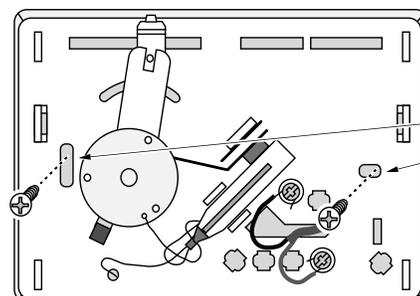
Attach the thermostat to the wall through these two holes.
