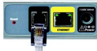
Figure 3-3: Connect to the LINE Port
