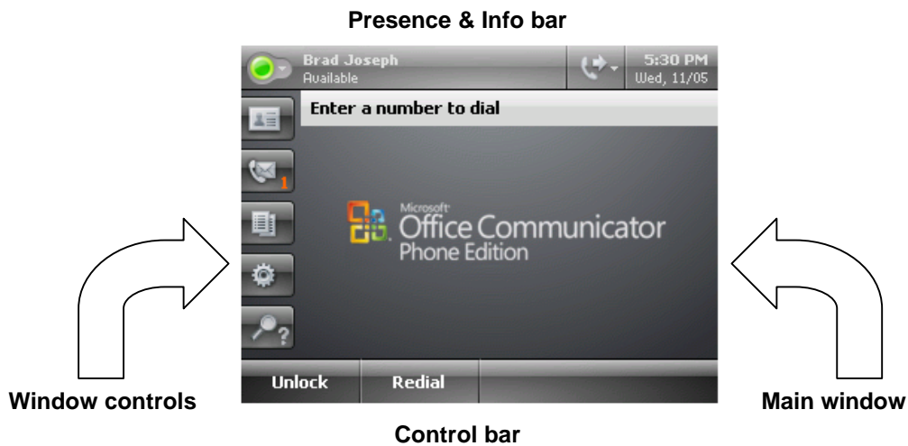
Figure 7: IP8540 screen layout
