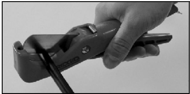
Figure 49: Cutting the Cable
