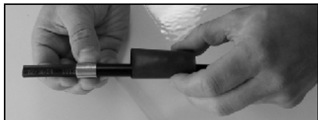
Figure 51: Placing the Heat Shrink Tubing and Ferrule
