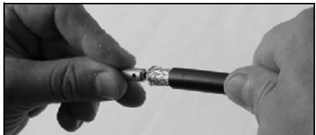
Figure 56: Deburring the Center Conductor
