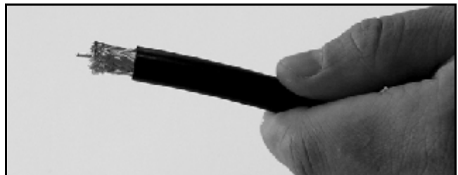
Figure 55: Cable Stripped, Exposing Dielectric
