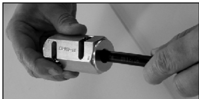
Figure 52: Stripping the End to Expose the Center Conductor
