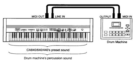
When connected as shown in the illustration, you can not only play along with the rhythm from the drum machine, you can also play the drum machine by striking the keys on the digital piano.
