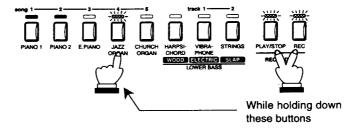
To cancel deletion, press the SONG button again so that the LED lights before releasing the PLAY/STOP and REC buttons.
