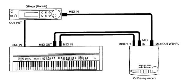
When connected as shown in the illustration, you can record songs played on the digital piano with the sequencer and play them back as many times as you like, and layer the module's tones made with the digital piano's MULTI TIMBRE function to assemble a complex automatic performance.
