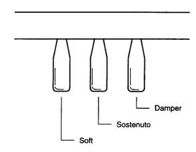
**Damper pedal:** Pressing this pedal sustains the sound even after removing the hands from the keyboard.
