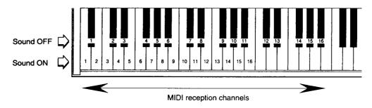
Use the 16 white keys at the left end of the keyboard to set the channels to ON. Use the 16 black keys at the left end of the keyboard to set the channels to OFF.
