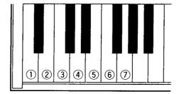
Volume is set to its lowest with the "1" key and at its highest with the "7" key. The "4" key is the factory setting.
