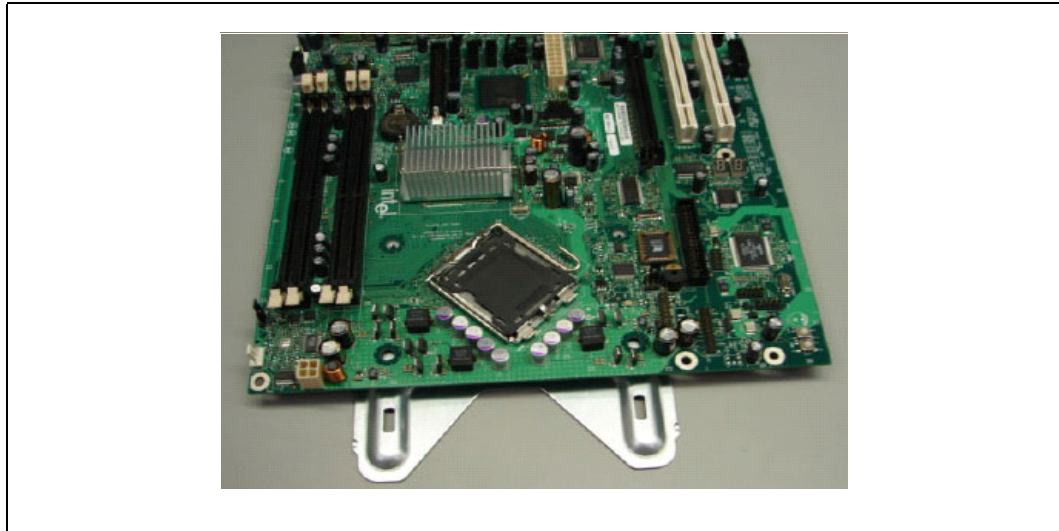
Figure 20. BTX board alignment on SRM
