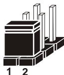
Jumper Block 1-2 pin close(enabled) Looks like this
