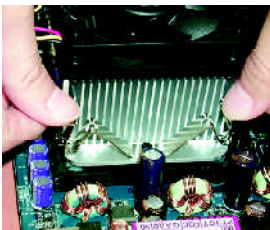
Figure 2. Fasten the cooling fan supporting-base onto the CPU socket on the motherboard.
