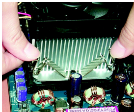
Figure 2. Fasten the cooling fan supporting-base onto the CPU socket on the motherboard.
