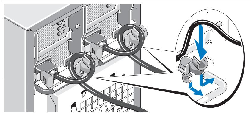
Attach the power cord retention bracket on the right bend of the power supply handle. Bend the system power cable into a loop as shown in the illustration and attach to the bracket's cable clasp. Repeat the procedure for the second power supply.
