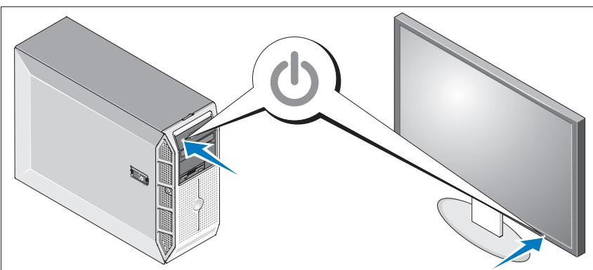
Press the power button on the system and the monitor (optional). The power indicators should light. Adjust the monitor's controls until the displayed image is satisfactory.
