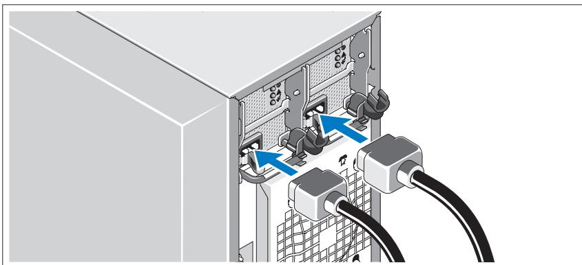
Connect the monitor's power cable to the monitor (optional), and connect the system's power cable(s) to the system.
