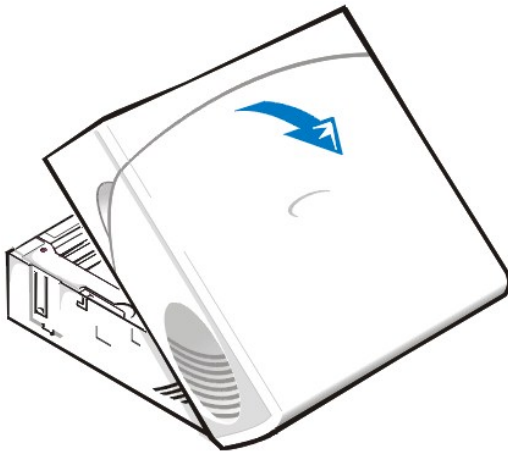
Figure 2. Removing the Low-Profile Computer Cover
