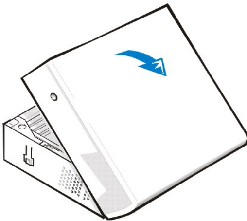
Figure 2. Removing the Low-Profile Computer Cover
