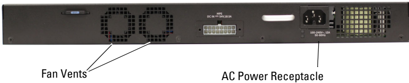
Figure 3-7. Dell EMC Networking N1500 Series Back Panel
