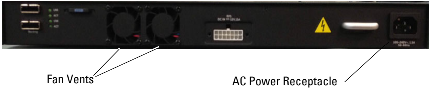
Figure 3-11. Dell EMC Networking N2000 Series Back Panel
