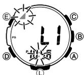
During manual receive, the signal level indicator displays the signal level as shown below.
