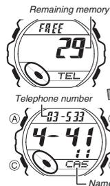
Telememo lets you store up to 30 records, each containing name and telephone number. Records are automatically sorted based on the characters of the name. You can recall records by scrolling through them on the display.
