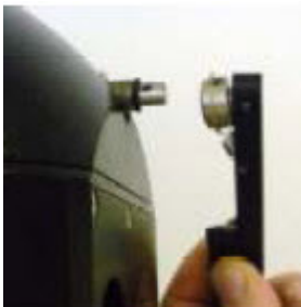
Figure 2.6: Remove Wiper Arm from wiper shaft
