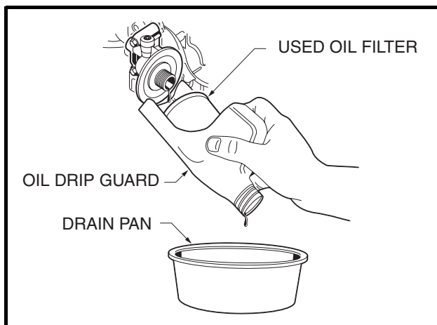
Figure 29 Remove Engine Oil Filter
