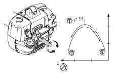
**CAUTION!** If the shaft is moving when the engine is idling the idle adjustment screw T should be turned anti-clockwise until the cutting attachment stops.
