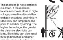
insulated. If the machine touches or comes close to highvoltage power lines it could lead to death or serious bodily injury. Electricity can jump from one point to another by arcing. The higher the voltage, the greater the distance electricity can jump. Electricity can also travel through branches and other objects, especially if they are
