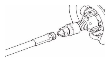
Screw the shaft using the nut and then using the fixed keys, tihgt them strongly.
